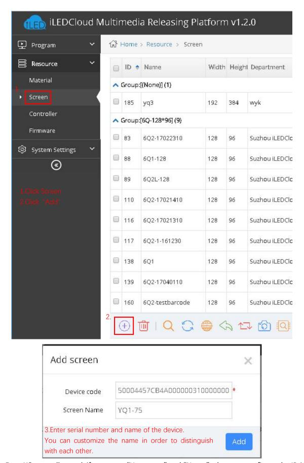
For a YQ controller card, if you enter "Username" and "Name" when you configure the IP, it will be automatically added under the corresponding user's account, otherwise it needs to be manually added. We recommend you to use bar code as serial number. Use identification code
