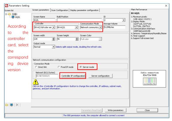
Choose "Server Mode" from "Wifi Mode", and then click "Controller IP Configuration". In the IP configuration interface, enter controller IP. Server IP: 139.196.231.196; Port: 3801. Then click "Setup" button. (Remark: Only one device can be connected in your local area network when you configure IP.)
